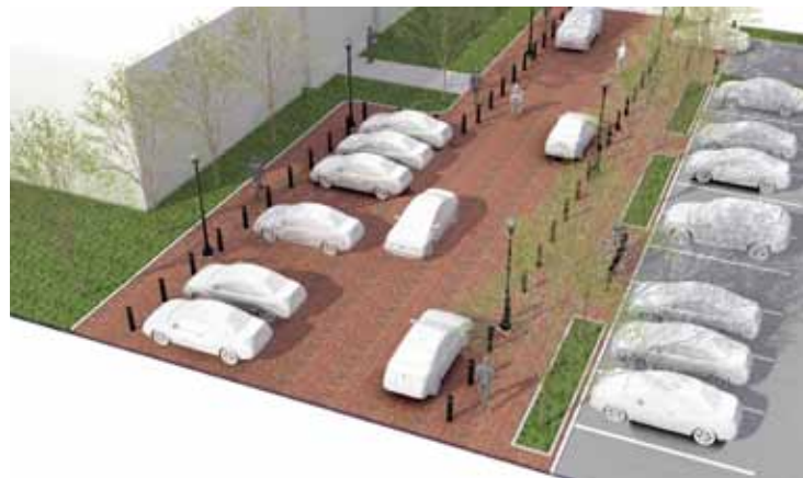
ALTERNATIVE CONCEPT DETAIL 2 - PEDESTRIAN WALKWAYS FLUSH WITH ALLEY, SEPARATED BY DECORATIVE BOLLARDS
