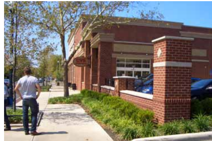
PARKING LOTS SHOULD BE SCREENED WITH A COMBINATION OF LANDSCAPE AND ARCHITECTURAL SCREENING
