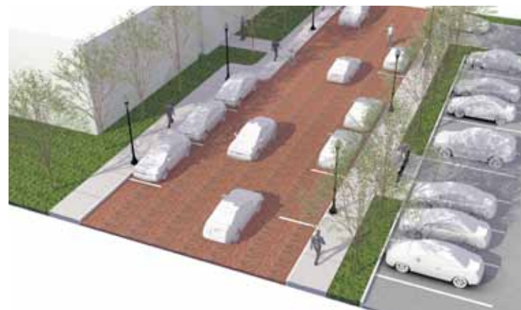
ALTERNATIVE CONCEPT DETAIL 3 - PARALLEL PARKING WITH RAISED SIDEWALKS ON BUILDING AND PARKING SIDES OF ALLEY
